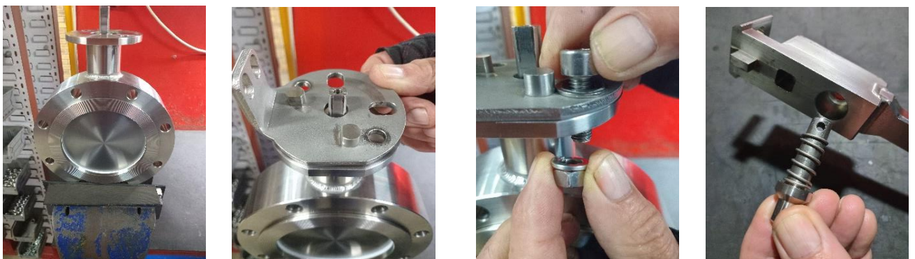
17 - 21 Fitment of main body, PTFE seal ring, PTFE seal insert and cover plate
