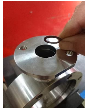
1 - 4 Fitment of Bottom Shaft & Grub screw
