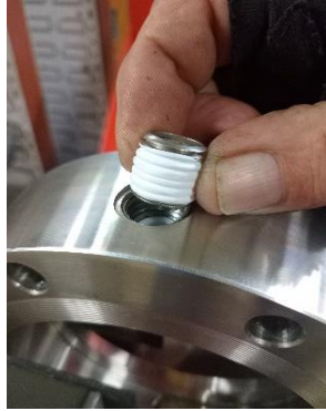
1 - 4 Fitment of Bottom Shaft & Grub screw
