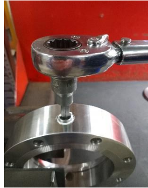
1 - 4 Fitment of Bottom Shaft & Grub screw
