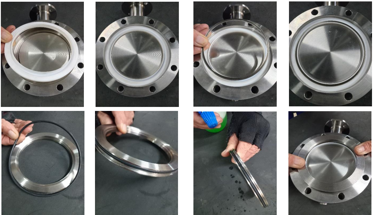
17 - 21 Fitment of main body, PTFE seal ring, PTFE seal insert and cover plate
