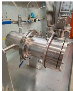
Test 1: Seat Tightness @ 27kPa for 5 minutes
