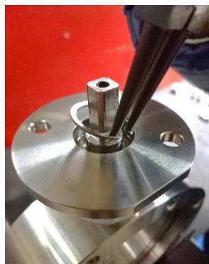
5 - 11 Fitment of Top Shaft & Circlip
