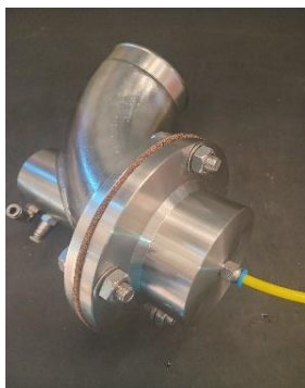
Test 1: Seat tightness @ 5,5kPa
