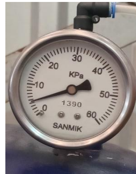
Test 1: Seat tightness @ 5,5kPa
