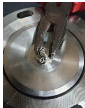
1 - 12 Main body assembly, piston, spring, spring retainer and sealing disc
