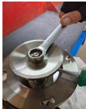
1 - 12 Main body assembly, piston, spring, spring retainer and sealing disc
