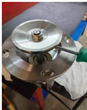
1 - 12 Main body assembly, piston, spring, spring retainer and sealing disc
