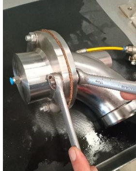
Test 1: Seat tightness @ 5,5kPa
