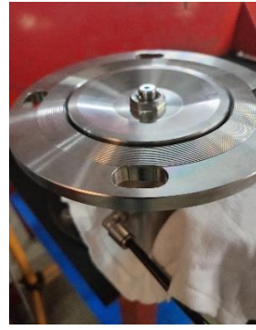
Operability testing opening/closing of main piston
