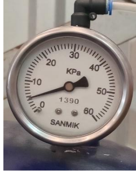
Test 1: Seat tightness @ 5,5kPa
