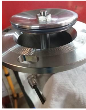
Operability testing opening/closing of main piston
