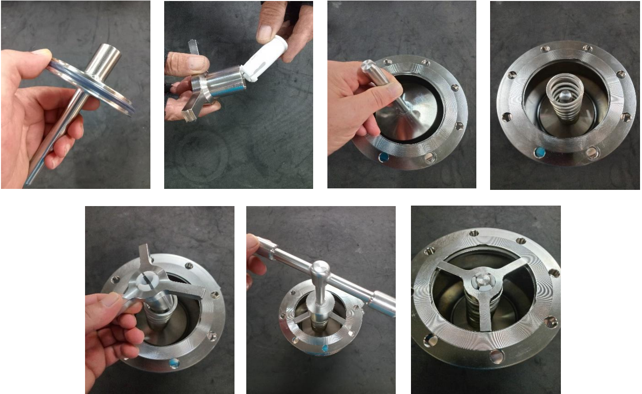
1 - 5 Sealing disc, spider and main body assembly
