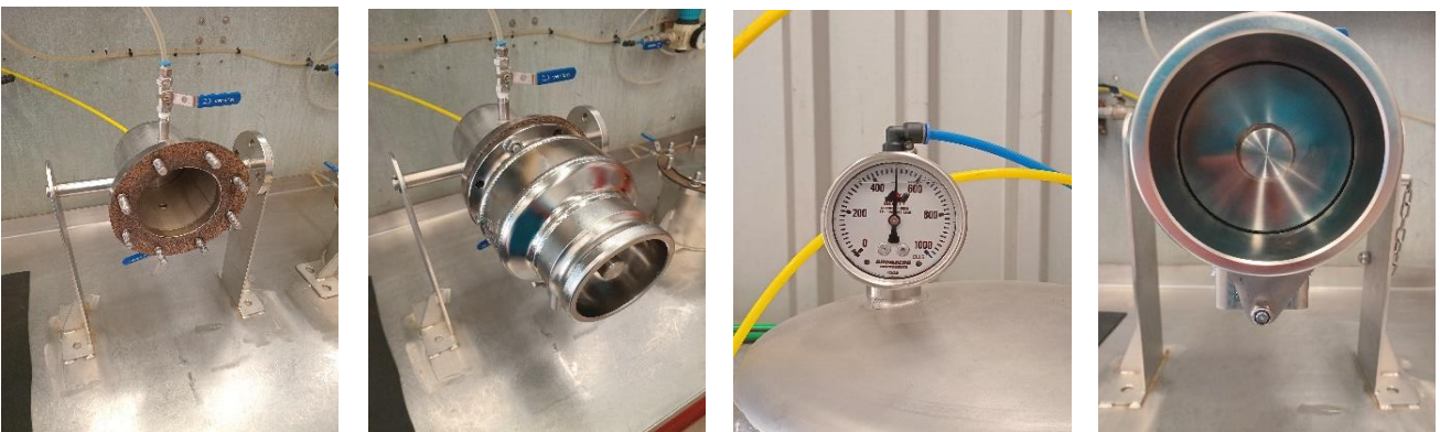
Test 2: Shell tightness @ 500kPa and Seat tightness @ 500kPa
