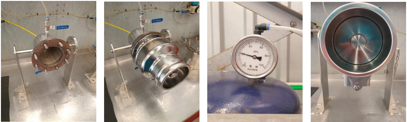
Test 1: Seat tightness @ 20kPa
