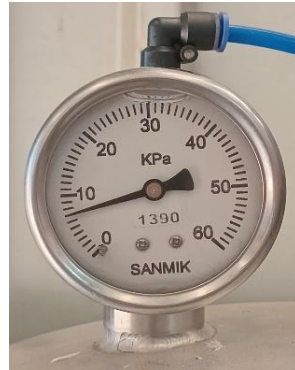
Test 1: Seat Tightness @ 7kPa
