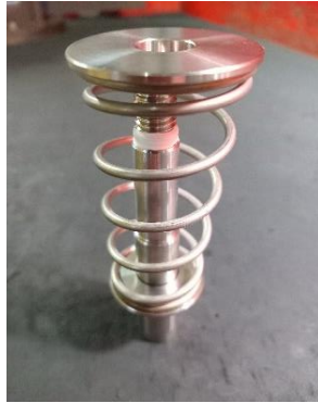
1 - 3 sealing disc rod, top spring guide, spring and bottom spring guide
