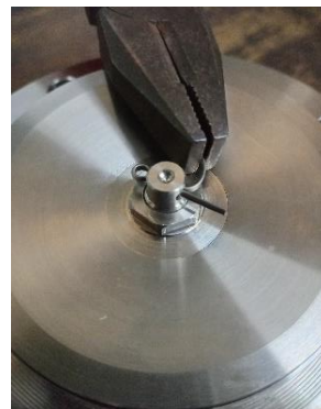
4 - 9 main body, sealing disc assembly, spring top and bottom retainer and spring
