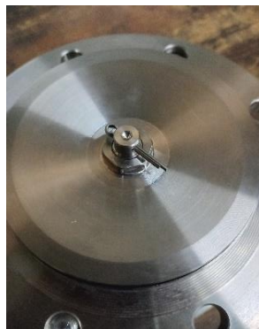
4 - 9 main body, sealing disc assembly, spring top and bottom retainer and spring
