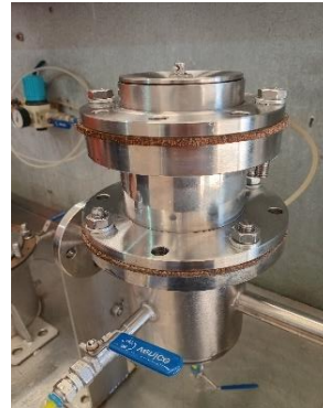
Test 1: Seat Tightness @ 7kPa
