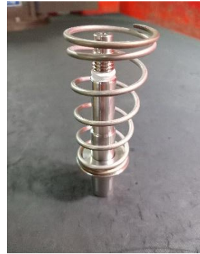
1 - 3 sealing disc rod, top spring guide, spring and bottom spring guide
