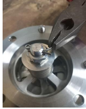
5 - 8 main body, sealing disc assembly, spring top and bottom retainer and spring
