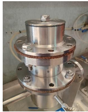
Test 1: Seat Tightness @ 27kPa
