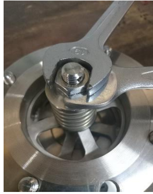
5 - 8 main body, sealing disc assembly, spring top and bottom retainer and spring
