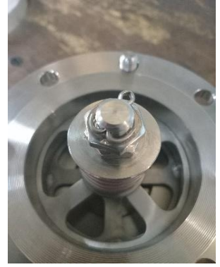
5 - 8 main body, sealing disc assembly, spring top and bottom retainer and spring
