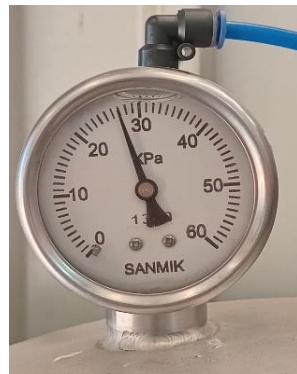
Test 1: Seat Tightness @ 27kPa
