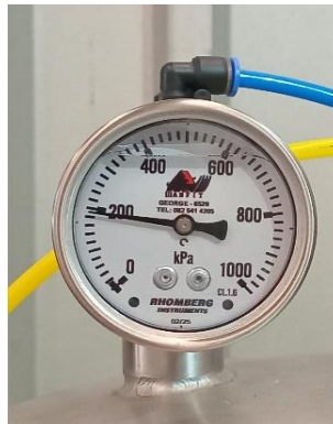
Test 1: Seat tightness @ 200kPa
