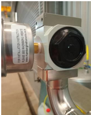
Test 1: Seat tightness @ 200kPa
