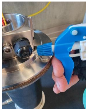
Test 2: Seat tightness @ 200kPa
