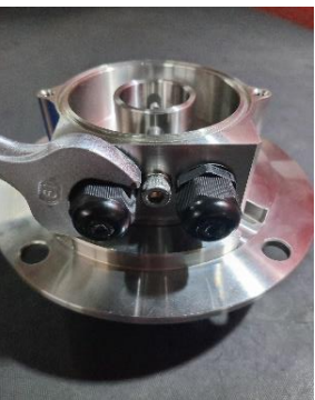
1 - 8 Quick Release Flange, Dixon Tube Housing body, Dixon Optic and Sealing Bush
