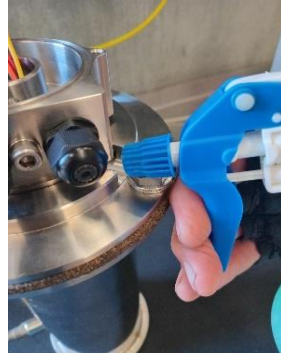
Test 1: Seat tightness @ 20kPa
