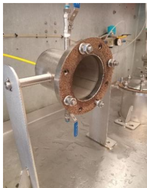
Test 1: Seat tightness @ 20kPa
