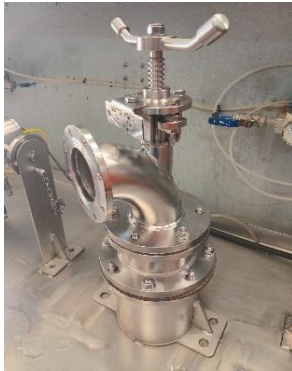
Test 1: Seat tightness @ 20kPa
