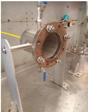
Test 1: Seat tightness @ 20kPa
