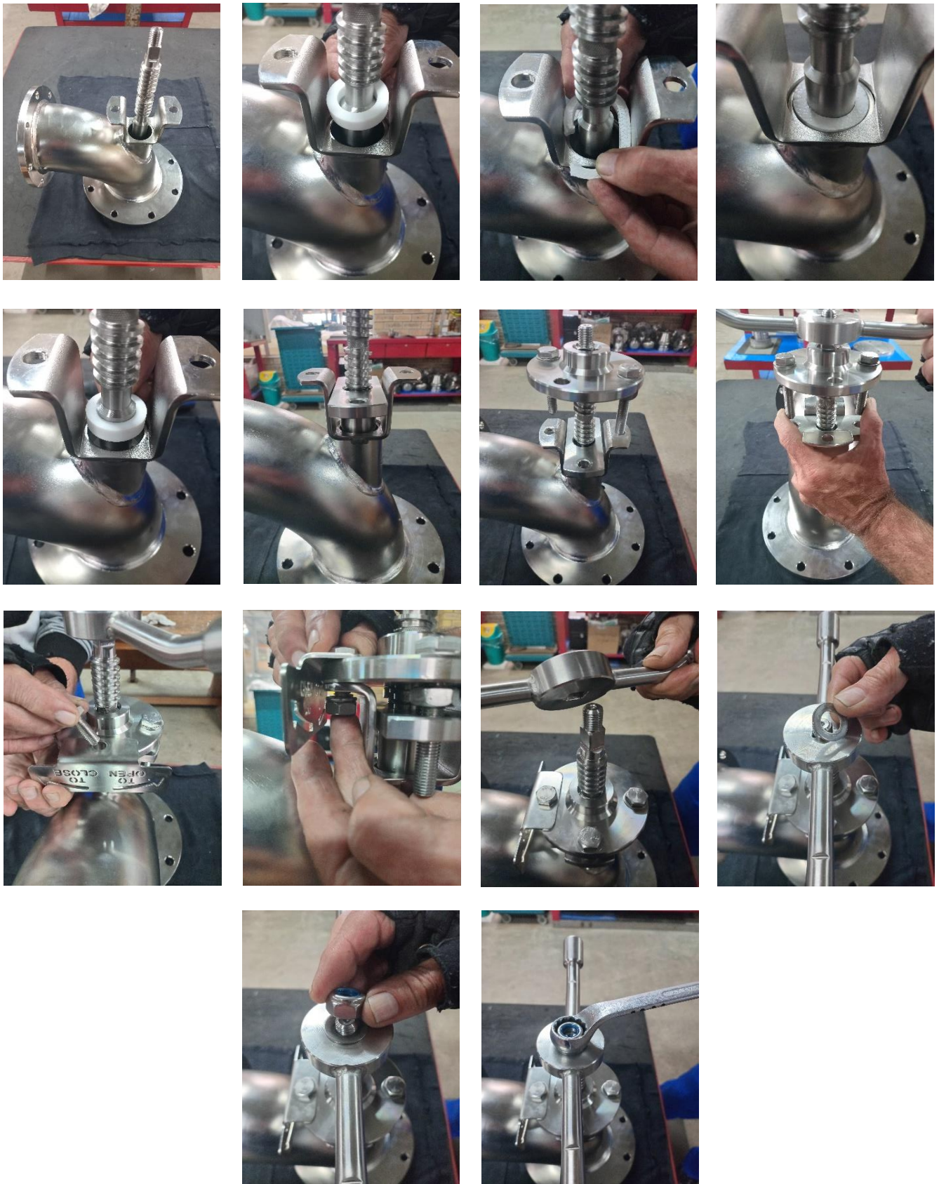
6 - 10 Main body, spindle assembly, top gland and spindle nut assembly (see parts assembly drawing for parts configuration)
