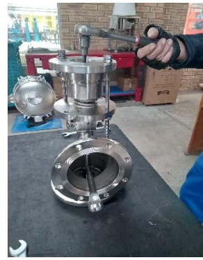
18 - 20 Main body and actuator assembly
