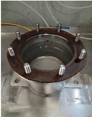
Test 1: Seat tightness @ 20kPa
