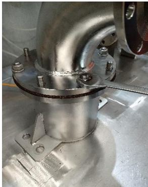
Operability testing opening/closing of sealing disc
