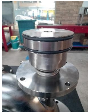
18 - 20 Main body and actuator assembly
