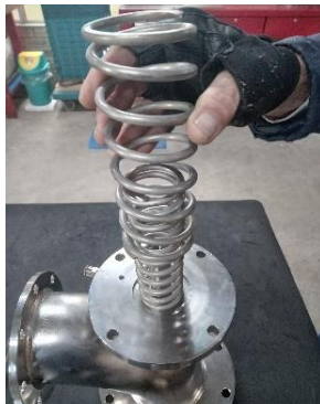
16 - 17 Main body and spindle flange assembly
