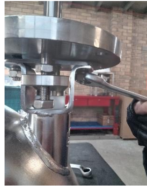
16 - 17 Main body and spindle flange assembly
