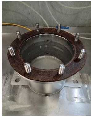
Test 1: Seat tightness @ 20kPa
