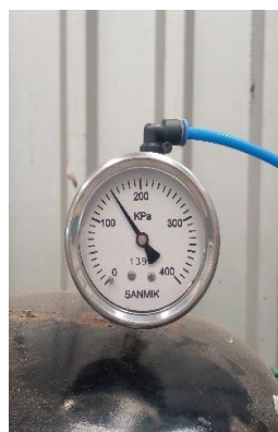
Test 1: Shell tightness @ 150kPa
