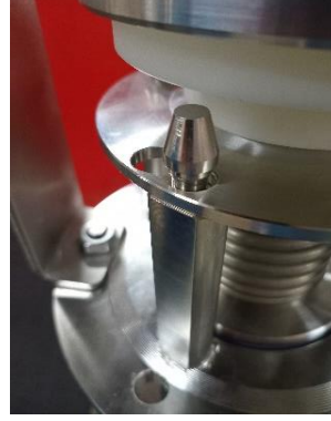
14 - 22 Main body, main piston, spring and cage assembly
