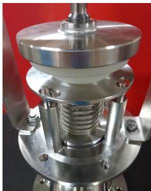
14 - 22 Main body, main piston, spring and cage assembly
