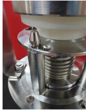
14 - 22 Main body, main piston, spring and cage assembly
