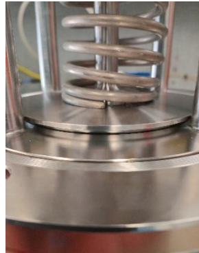
Test 1: Shell tightness @ 500kPa and Seat tightness @ 500kPa
