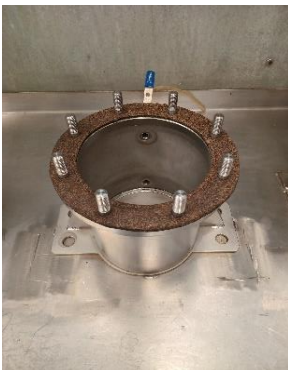
Test 2: Seat tightness @ 27kPa
