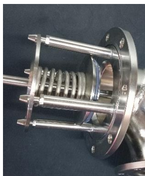
Operability testing opening/closing of main piston
