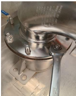
Test 1: Shell tightness @ 500kPa and Seat tightness @ 500kPa
