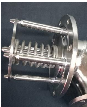
Operability testing opening/closing of main piston
