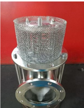
Test 2: Seat tightness @ 27kPa
