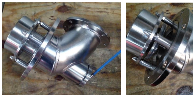
Test 1: Operability testing opening/closing of main piston
