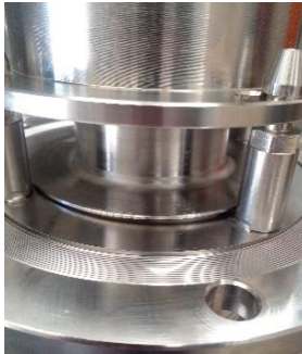
Test 2: Shell tightness @ 500kPa and Seat tightness @ 500kPa
