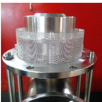
Test 3: Seat tightness @ 27kPa
