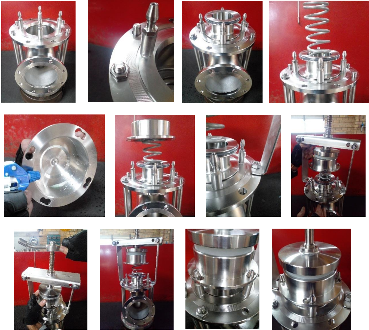
15 - 25 Main body, main piston, spring and cage assembly
