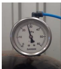
Test 3: Seat tightness @ 27kPa
