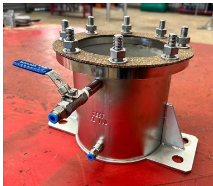
Test 2: Shell tightness @ 500kPa and Seat tightness @ 500kPa
