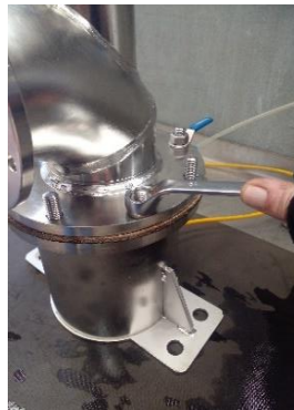
Test 2: Shell tightness @ 500kPa and Seat tightness @ 500kPa
