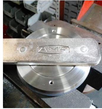
2 - 6 Sealing Disc Assembly
