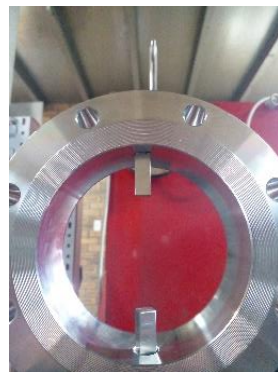
13 - 16 Fitment of Bottom Shaft & Grub screw
