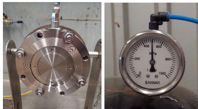
Test 2: Seat Tightness @ 500kPa for 5 minutes
