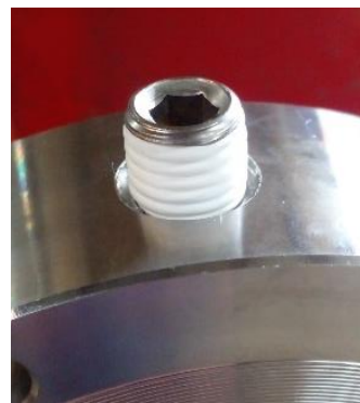
13 - 16 Fitment of Bottom Shaft & Grub screw
