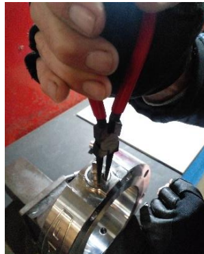
7 - 12 Fitment of Top Shaft & Circlip
