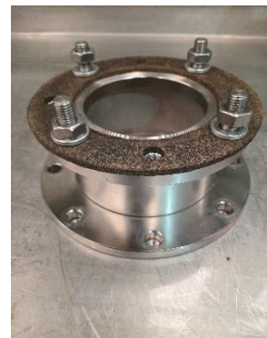
Test 1: Seat Tightness @ 20kPa for 5 minutes
