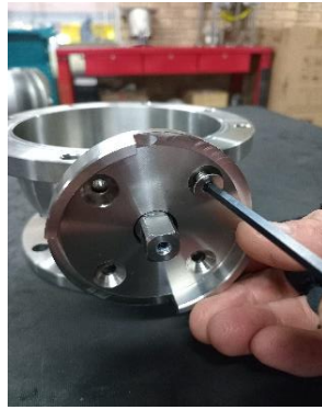
1 - 6 Main body (Long), shaft and shaft plate assembly
