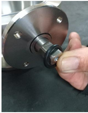
1 - 6 Main body (Long), shaft and shaft plate assembly
