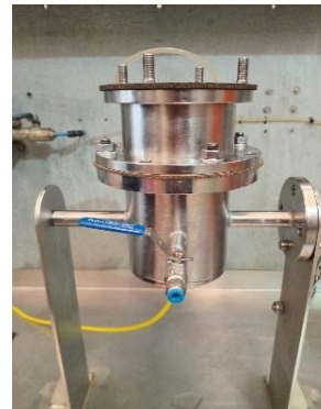
Test 1: Seat Tightness @ 20kPa for 5 minutes
