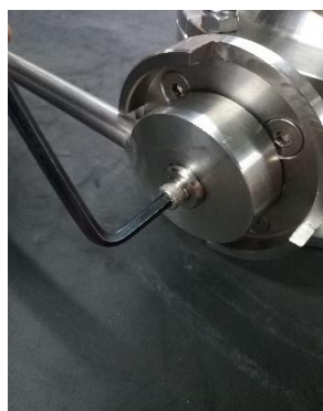
7 - 12 Main body, ball and handle assembly
