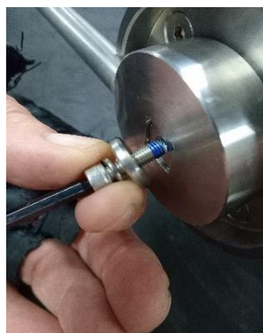
7 - 12 Main body, ball and handle assembly
