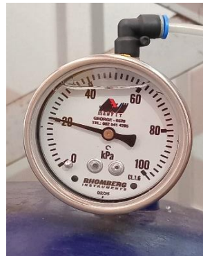
Test 1: Seat Tightness @ 20kPa for 5 minutes
